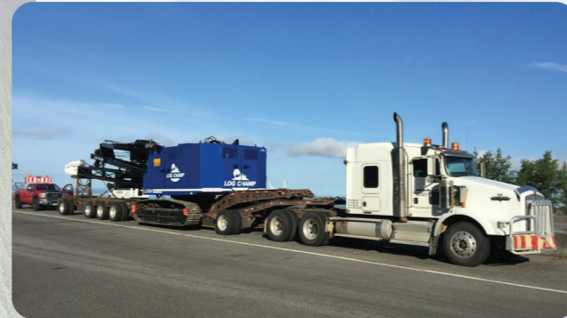
Easy relocation with a self folding boom and gantry, power tilting cab on both models. In addition the 550 can be moved in a single load.
