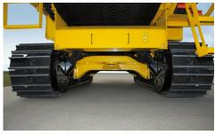
MOBILITY. The track-driven grinder offers onsite mobility with a remote control. The HG4000TX is designed with 16" (40.6 cm) of ground clearance, enhancing the unit's ability to traverse difficult
