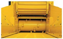
**OPTIMAL CUTTING PERFORMANCE.** The duplex drum offers proven cutting performance, and reversible hammers and tips nearly double the wear life of single-sided designs and simplify daily maintenance. The optional chip drum produces a consistently chipped end product, rather than traditional shredded material, for uses such as biofuel.
