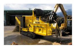
PROGRESSIVE PROCESSING. The patented SmartFeed system monitors engine rpm and adjusts grinding speed to increase productivity. The open-ended, wide infeed table makes material loading easy and efficient.
