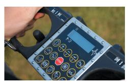
**REMOTE CONTROL.** A state-of-the-art wireless remote control unit allows the operator to run most machine functions from up to 300' (91.4 m) away.
