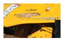
PATENTED SMARTSWEEP® CUTTER SYSTEM. The patented SmartSweep® control system monitors engine speed and automatically adjusts cutterwheel sweep rate to maximize power to the cutter wheel while reducing engine stress.
