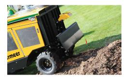
MOVE CHIPS AROUND THE JOBSITE. In narrow jobsite conditions that restrict use of the main control station, the operator can control ground drive and steering functions from this folding station mounted at the front end of the machine.
