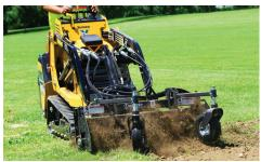
**BUILT TO PERFORM.** Get more out of each day with a tipping capacity of 2643 lb (1198.8 kg) and rated operating capacity of 925 lb (419.6 kg) while reaching to maximum hinge pin height at 84.5" (214.6 cm).
