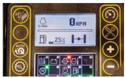
KNOWLEDGE ON DISPLAY. An integrated system display toggles through machine diagnostics, including engine rpm, fuel, battery voltage, engine water temperature and engine hours. When in either ground drive or using a rear attachment, the display indicates the percentage of the hydrostatic capacity being utilized, allowing the operator to easily monitor important machine functions.
