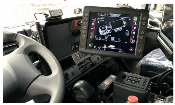
The Gen 6 Bucher iQ CANBus Control System comes complete with a fully integrated 12" Touch screen providing the operator with the latest technology and user interface for ease of operation. Designed in collaboration with Bucher Engineers, the new touch screen monitor replaces the previous push button control console and provides access to all body/compaction functions and system maintenance through the one screen.
