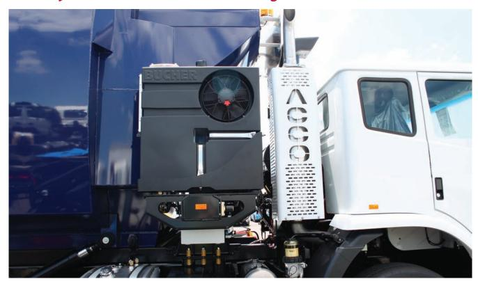
The SPORT Gen 6 has a new and improved Hydraulic Oil Tank and Cooling Package to provide efficient and low cost operation.
