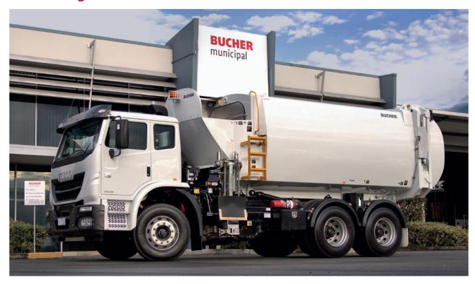
Bucher Municipal is proud to introduce the Xtreme Side Loader, providing extreme Maneuverability, Payload, Safety, Bin lifter Reach and Productivity. With its short 4400mm wheelbase and compact body design, the Xtreme Side Loader can provide 10T payloads in the most compact 6x4 chassis configuration achievable.
