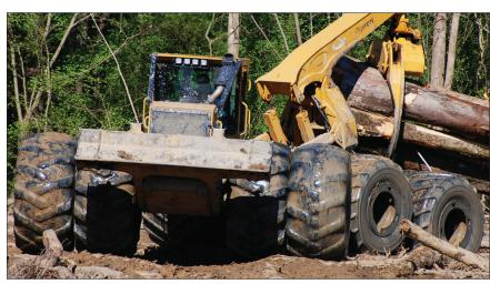
All models are standard equipped for dual or flotation tires.
